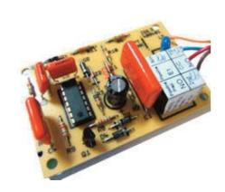
A feature that some boilers require, pump overrun is when the boiler pump continues to run after the boiler has finished firing.
